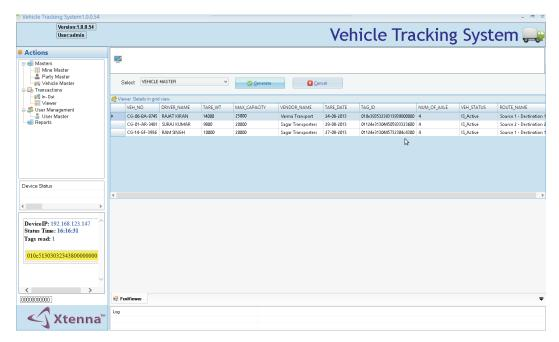
The vehicle log data for entry and exit displays the truck contractor's name (party name), the driver's name, vehicle license plate number, contracted period and the date, time and location of tag reading at the gate.
