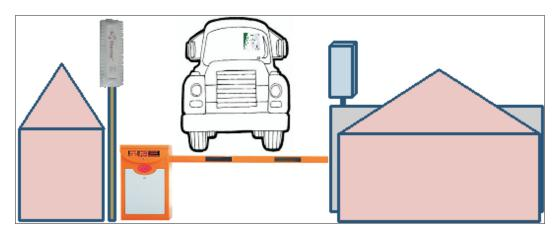
windshield of the truck and sends the tag details to the server. The system checks if the truck is registered in the database. If it finds the truck registered, it sends a command to the trigger switch that controls the boom barrier. The boom barrier is lifted, the truck is allowed to enter and its entry time is logged into the system.
