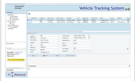
Individual truck details are registered in the Vehicle Master. These include the truck license plate number, driver name, contact number and address, etc. A PARKA™ RFID tag is read using the Xtenna Proximity™ reader and assigned to the vehicle in the database. The tag is then affixed on the truck's windshield. The truck owner (vendor/contractor) is selected from the previously entered screen and assigned to the vehicle in the database.
