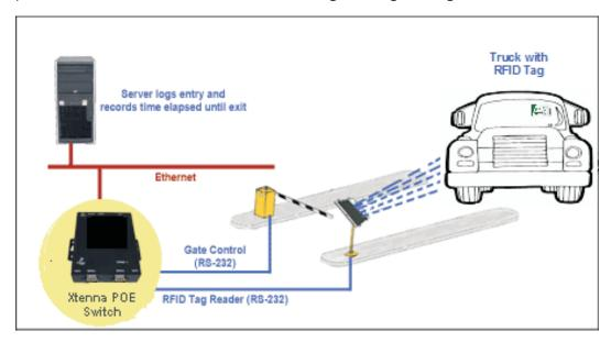
The Vehicle Tracking System displays alerts on screen if it detects an unregistered tag or if the tag indicates that the vehicle's contract period has expired and the truck driver is attempting entry after the valid date has lapsed.
