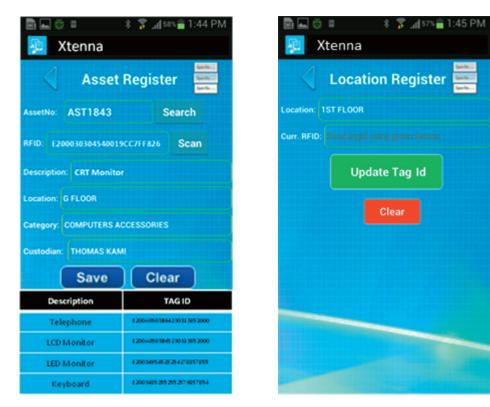
Location Register: The operator selects a location from the location list, then scans the METALLICA<sup>™</sup> tag affixed at that location using the HandyScanna<sup>™</sup> and saves the data into the device.
