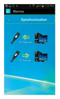
The operator then moves to the next location and repeats the process. After scanning at all locations has been completed, the local data of inventory audit is uploaded to the Server using the Synchronization function.
