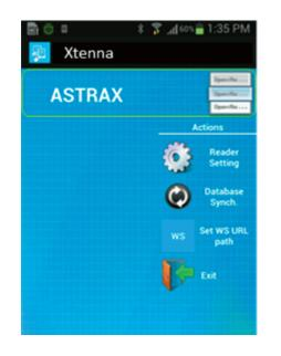
**Reader Setting:** This enables the user to set the read and write power of the HandyScanna<sup>™</sup> device, the region, and the antenna mode i.e. whether bistatic or monostatic, etc.
