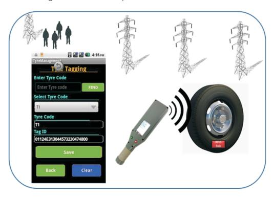
5. Next the tyres are assigned in the database to the vehicles to which they have been issued, including the spare tyres in the set. The hand-held screen indicates the number of tyres assigned to the vehicle.
