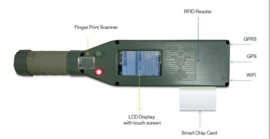
5. On successful completion, a receipt is generated with the tag ID, fertilizer type, GPS co-ordinates and the farmer's ID printed on it.
