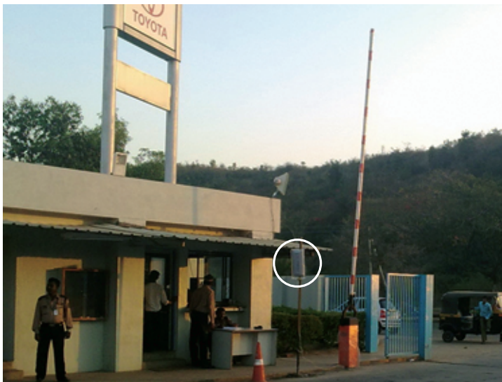
Xtenna™ Reader/ Antenna (shown circled in picture) deployed at gate
